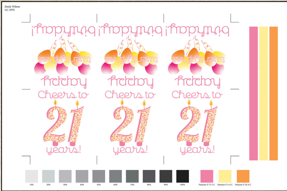
3-UP IMPOSITION OF CLIENT CARDS WITH TINT BOXES, REGISTRATION MARKS, AND COLOR BARS. COLORS USED: PANTONE P 73-5 C, PANTONE P 4-4 C, AND PANTONE P 24-6 C
