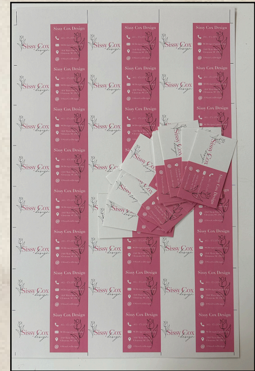
PRINTED 24-UP IMPOSITION CLIENT BUSINESS CARDS, TRIMMED AND UNTRIMMED. COLORS USED: PANTONE P 73-5 C AND PANTONE PROCESS BLACK
